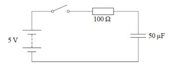
Describe what happens to the potential difference across the resistor and the potential difference across the capacitor after the switch is closed.
