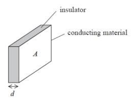
The capacitor has a capacitance 0.1  $\mu F$  and is charged to a p.d. of 100 V by connecting it to an electrical supply.
