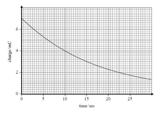
Calculate the capacitance of the capacitor.
