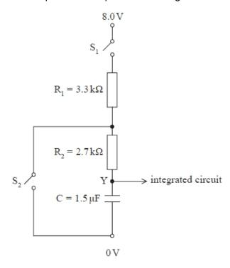
When the potential at Y is  $8.0\,V$ , the switch  $S_2$  is closed.
